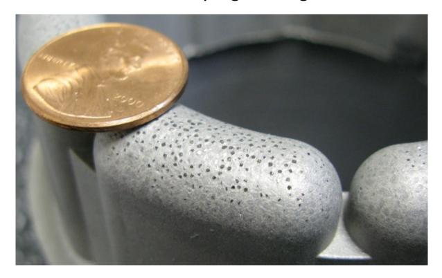
Our XDS burn shoes have a tungsten carbide matrix head that is impregnated with 30-40 mesh diamonds from the surface to about 1/2" deep into the shoe face. As work is done the diamond will be sloughed off as it dulls and fresh grit will be exposed to do work.
