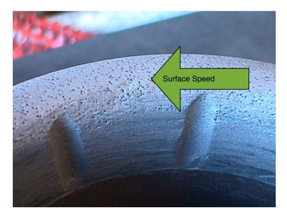
The shoe head has a valid cutting structure until this 1/2" is used up. This type of cutting structure has been used to cut hard steel, case hard steel, carbide, 13 chrome, inconel, as well as many softer components.
