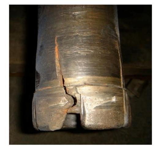
This XDS shoe was used on jointed pipe to burn over one plug with carbide slip buttons and then was used without rotating to push downward on the fish with 20,000 pounds which belled the shoe head. The internal failsafe mechanical locking of the worked so that only a small amount was lost downhole. XDS shoes are not intended to have such high forces transferred through them...especially when not rotating.
