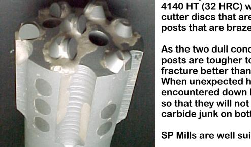
Economy Grade SP mills are steel bodied 4140 HT (32 HRC) with 10mm (3/8") PDC cutter discs that are mounted on 1/2" steel posts that are brazed deep into the mill face.
