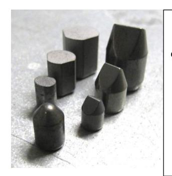
We can fabricate almost any shape of steel mill face and set it using either Low Torque cutters shown at left and the High Torque cutters shown at right. They are available in 1/2", 3/8", and 1/4"
