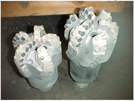
Right is a used 6 1/8" VZ-26 bit (Chevron Name Is OB-1A+) #CV-51011 run for Chevron on 5 oilbase Lobo wells to total 10,024 ft. @42.2 fph. The bit has been refit for rental use.
