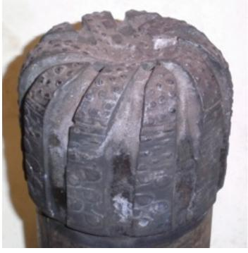
Second Run: Milled 22 frac ports total time 20 hrs and measured 1/4" under gage
