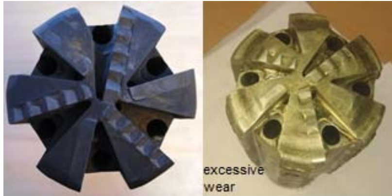
Before After TT Turbodrill mill before and after first run
