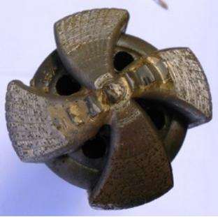
Second Run cut bottom part of Ball Valve in 4 hours
