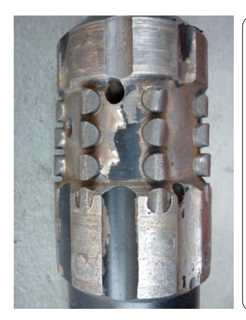
This SXR Reamer has a pilot diameter of 3.530" and three steps of .070" on diameter each out to 3.750". Using HPI (hot pressed impreg) inserts brazed into the steel body.
